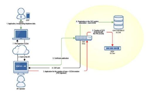
AC Camerfirma has a solution for the centralised key management system. The keys are created in an HSM FIPS 140 2 level three where they are stored for subsequent use by the public key certificate holders that are associated with them.
